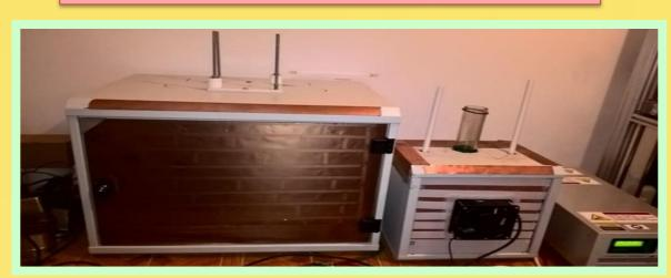
For RF treatment applying was used a 27.12 MHz RF Demonstrative laboratory model. The breads were packaged and heated at same temperature (75°C) applying RF treatment. Samples were incubated at 25°C and monitored for 10 days in order to establish the efficacy on the inhibition of fungi development.
