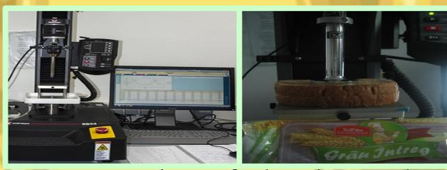
Texture properties of bread samples were measured with texture Analyzer Instron (model 5944, Illinois Tool Works Inc., USA), using a turntable compression diameter 40 mm at room temperature. With Bluehill 3.13, 4 texture parameters were calculated: fermity, elasticity, coesivity, gumosity.
